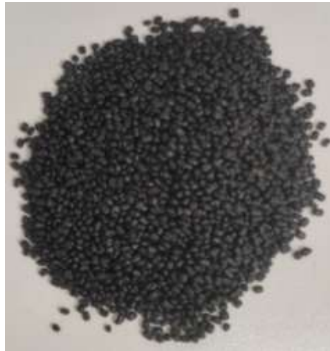
Seriplast compound 100% recycled FPP
